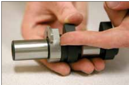
4. Make sure flange on decompressor is facing out
