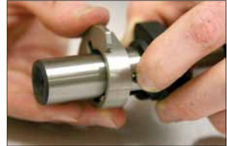
3. Hold spring in while sliding OEM decompressor over
