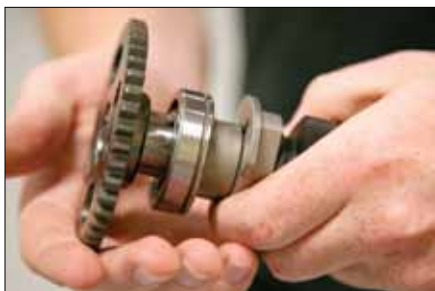
10. With teeth facing out, fit sprocket by hand with key still in place
