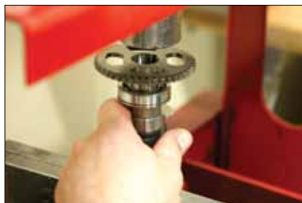
11. Using a press, press sprocket on to the cam
