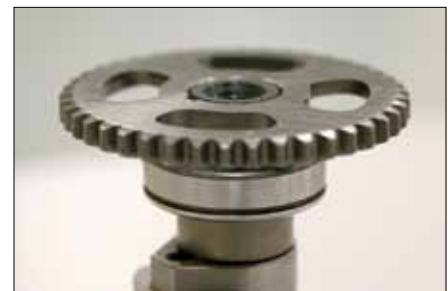
12. Continue to press sprocket until it is flush with the cam shaft
