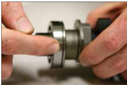
7. Make sure groove on bearing faces inward
